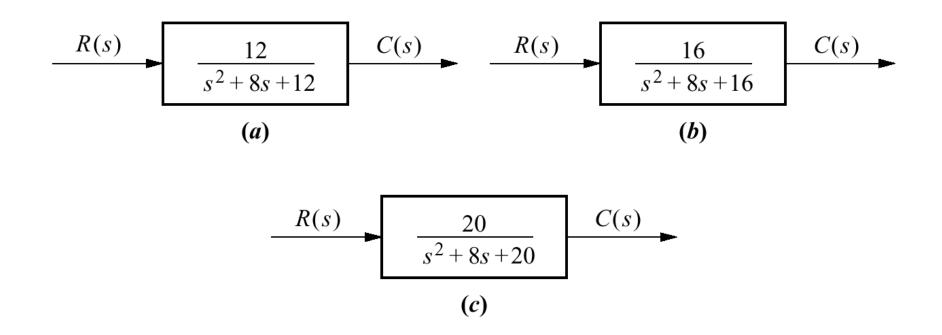
Figure 4.13 Second-order underdamped responses for damping ratio values
