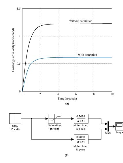
Figure 4.30 a. Effect of deadzone on load angular displacement response; b. Simulink block diagram
