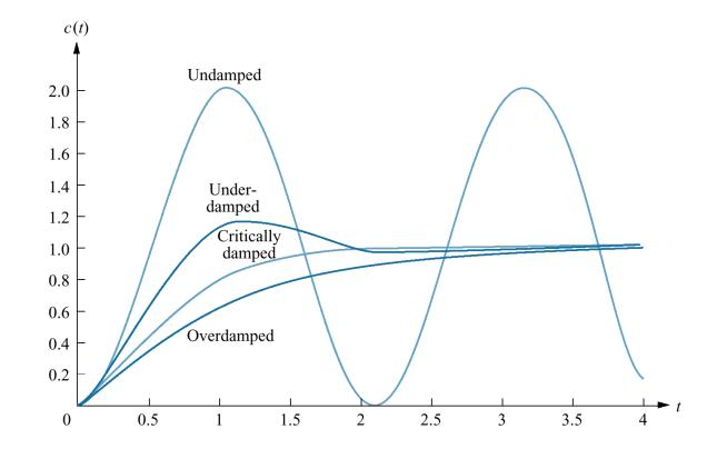
**Figure 4.11** Second-order response as a function of damping ratio
