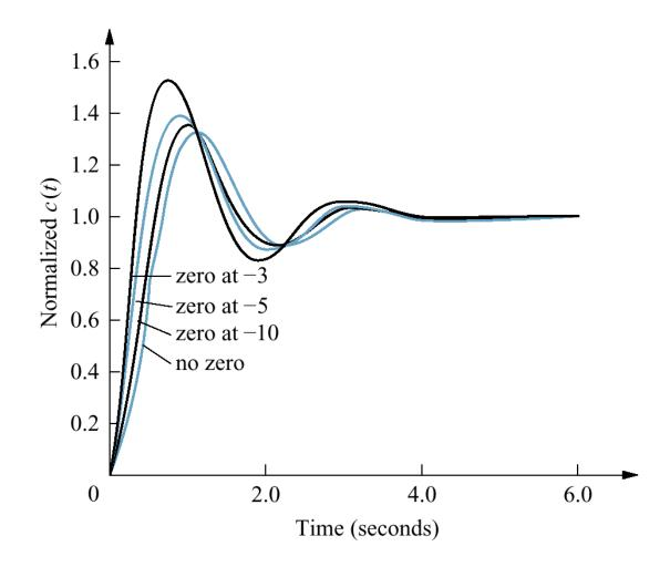
Figure 4.26 Step response of a nonminimum-phase system
