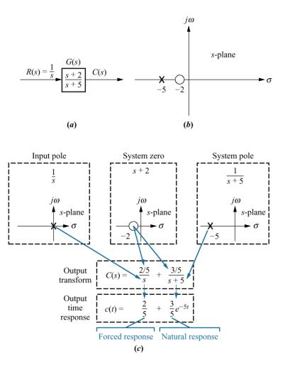
Figure 4.2 Effect of a realaxis pole upon transient response
