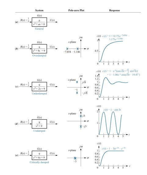
Figure 4.8 Second-order step response components generated by complex poles
