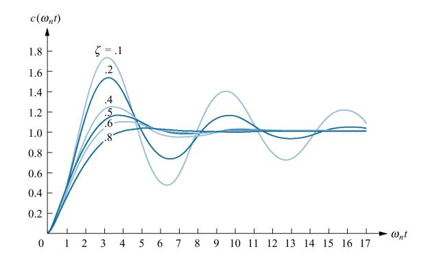
Figure 4.14 Second-order underdamped response specifications
