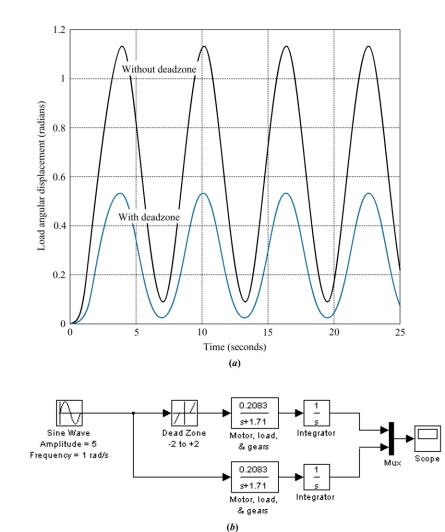
Figure 4.31 a. Effect of backlash on load angular displacement response; b. Simulink block diagram
