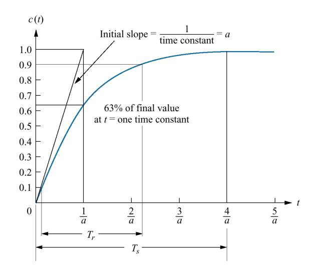
**Figure 4.6** Laboratory results of a system step response test
